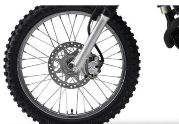
**Disc front brake and rear drum**
